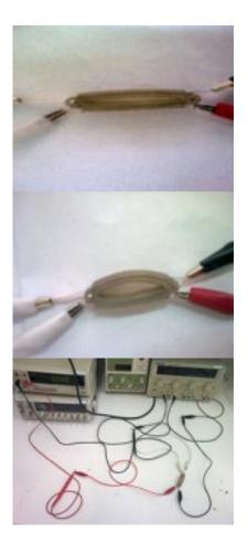
An artificial urinary sphincter made of two-way shape memory NiTi alloy embedded in silicon rubber is designed for prosthesis surgery in case of patients who suffer from urinary incontinence. The metallic part curves down when actuated by electrical current and straightens up when the current stops. This produces a smart composite for urination control in patients inflicted with spinal cord injury.
